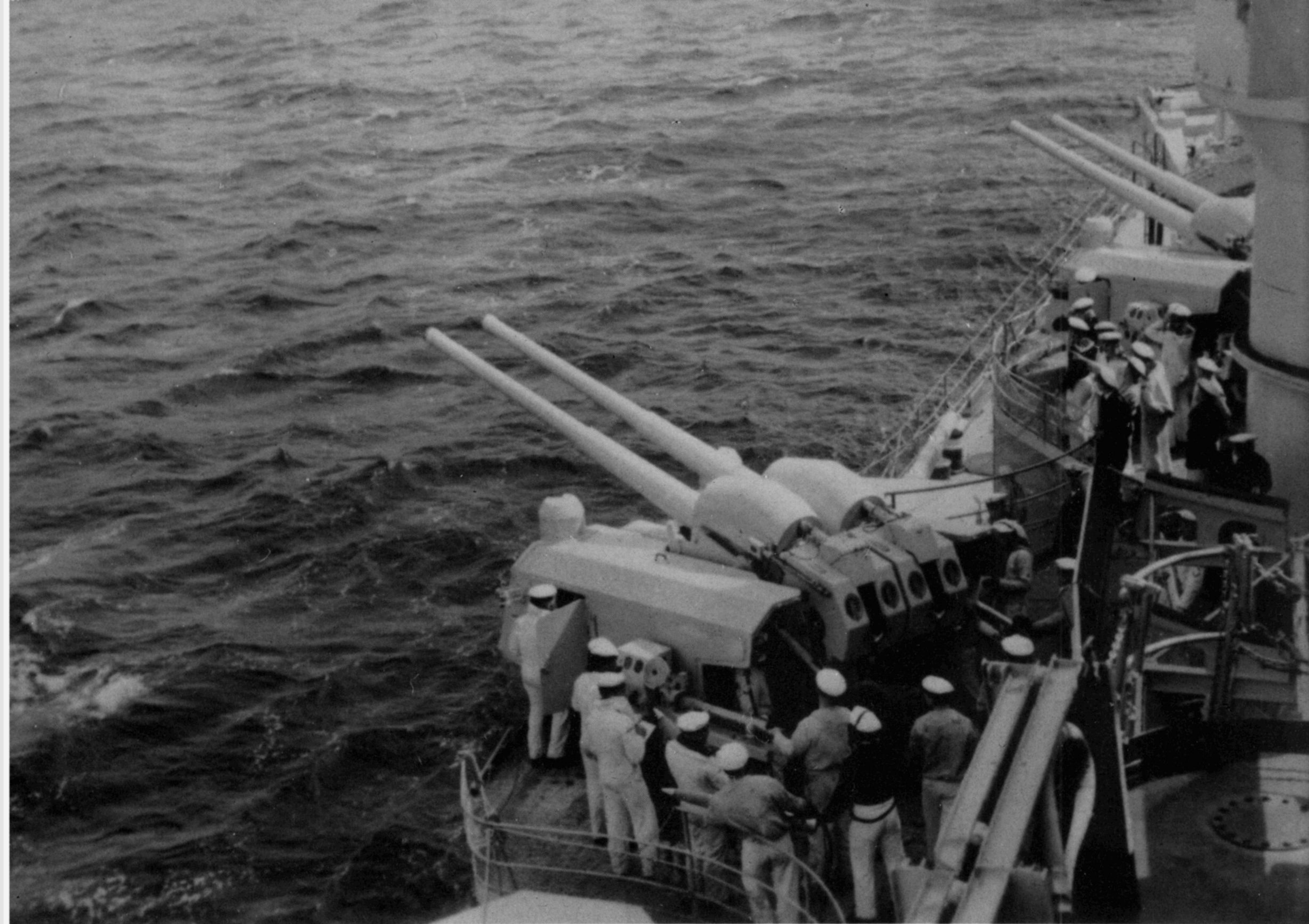
Two of the 105mm anti-aircraft guns grouped on the starboard side. The crew is performing firing drill. The picture was taken before the war began.
