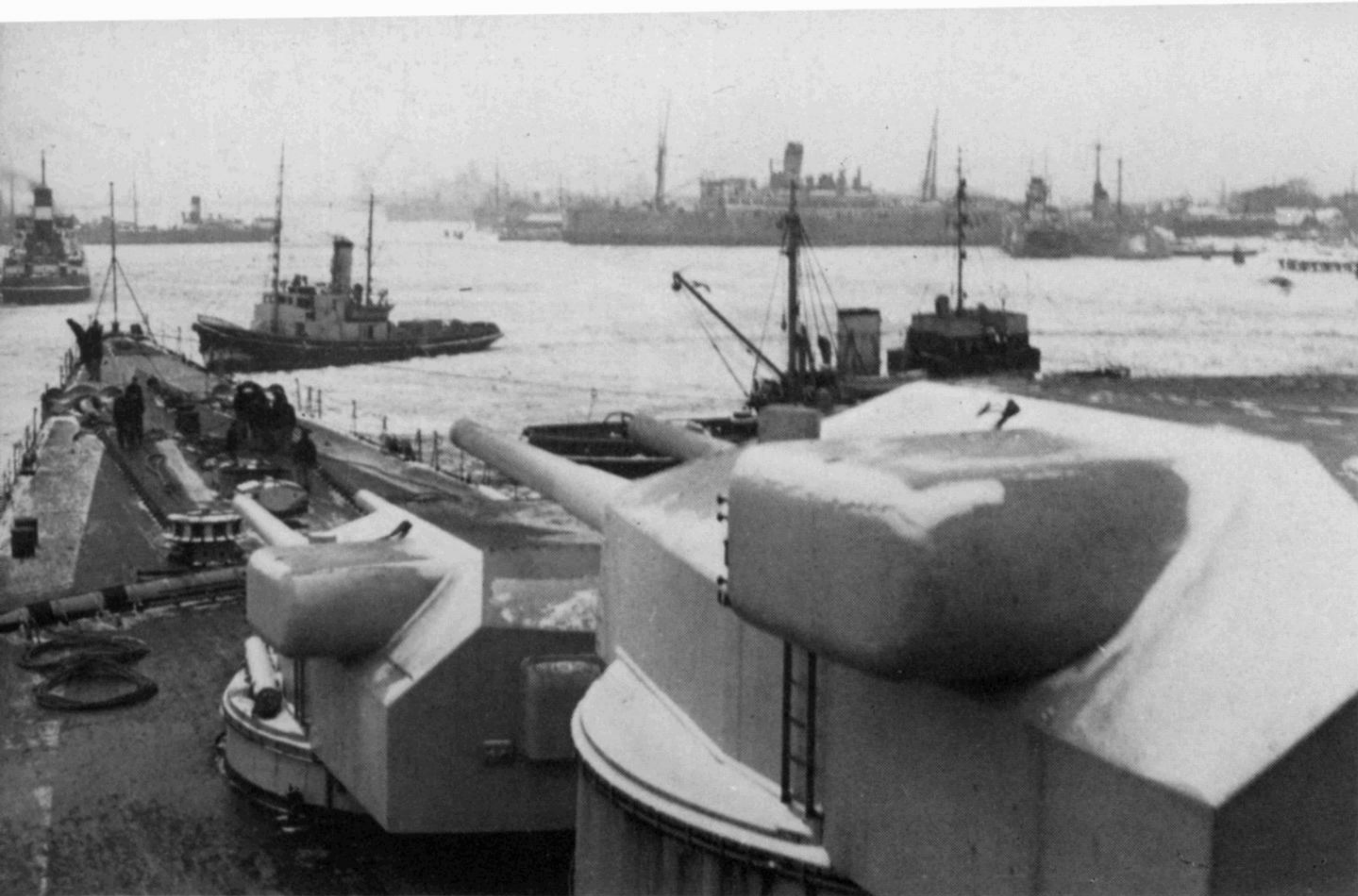
The forward 28-cm turrets. The left-side electric range finders on the turret sides can be seen clearly. This picture was taken early in 1940, under heavy ice conditions in Wilhelmshaven. In the far background (to the right of the large floating crane) is the sister ship GNEISENAU in a dock, farther to the right the cruise ship TANGANJKA of the Woermann Line of Hamburg, used as a barracks ship, and even farther right the target ship ZHRINGEN.
