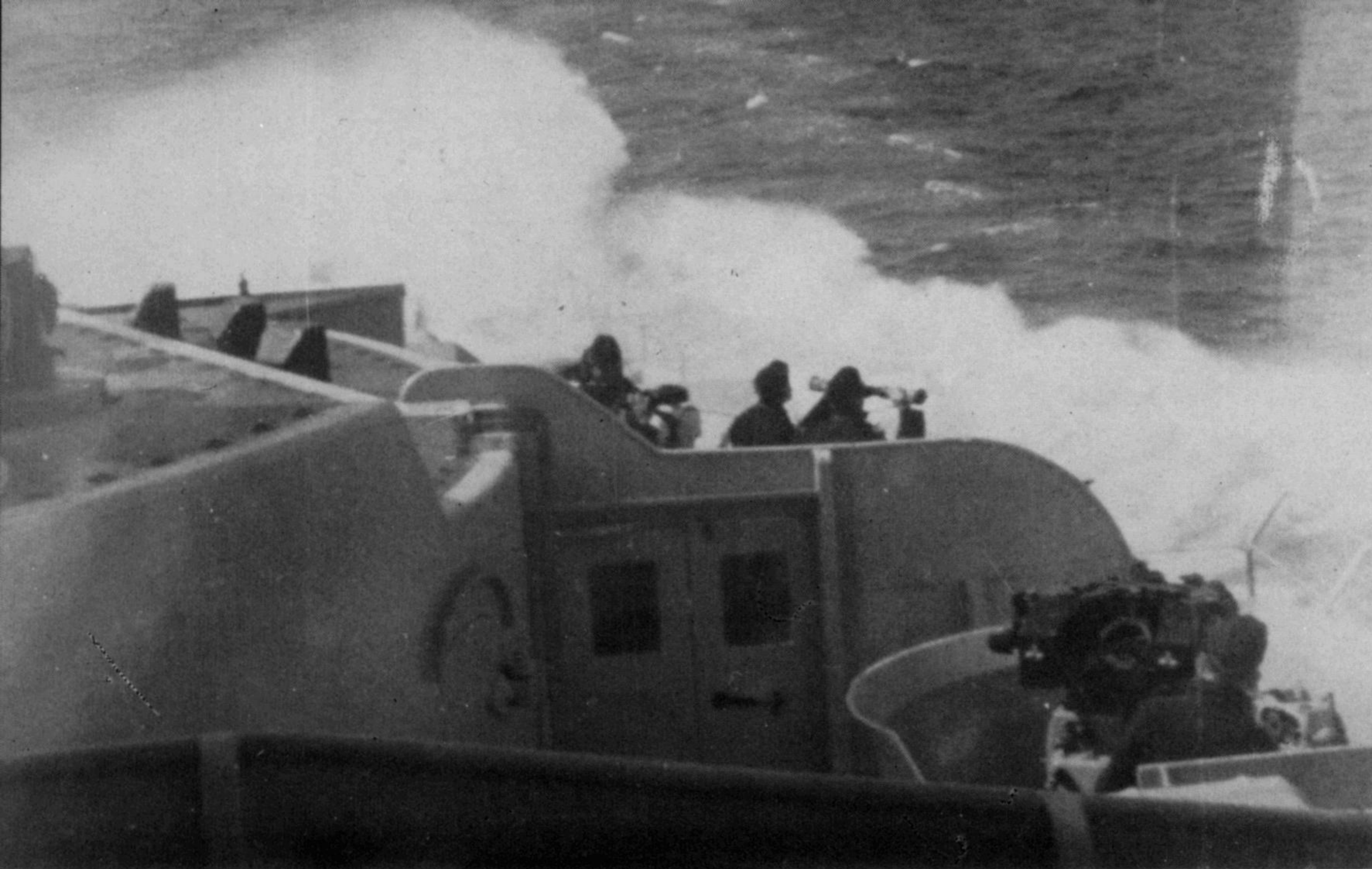
A look at the forward bridge structure. The SCHARNHORST holds a high speed, and the bow is covered with heavy spray. At the left edge of the picture is the forward command post, which was armored especially heavily. At right is a targeting device, behind it is a crewman at work with a small portable range finder. The picture may well have been taken during Operation "Berlin."
