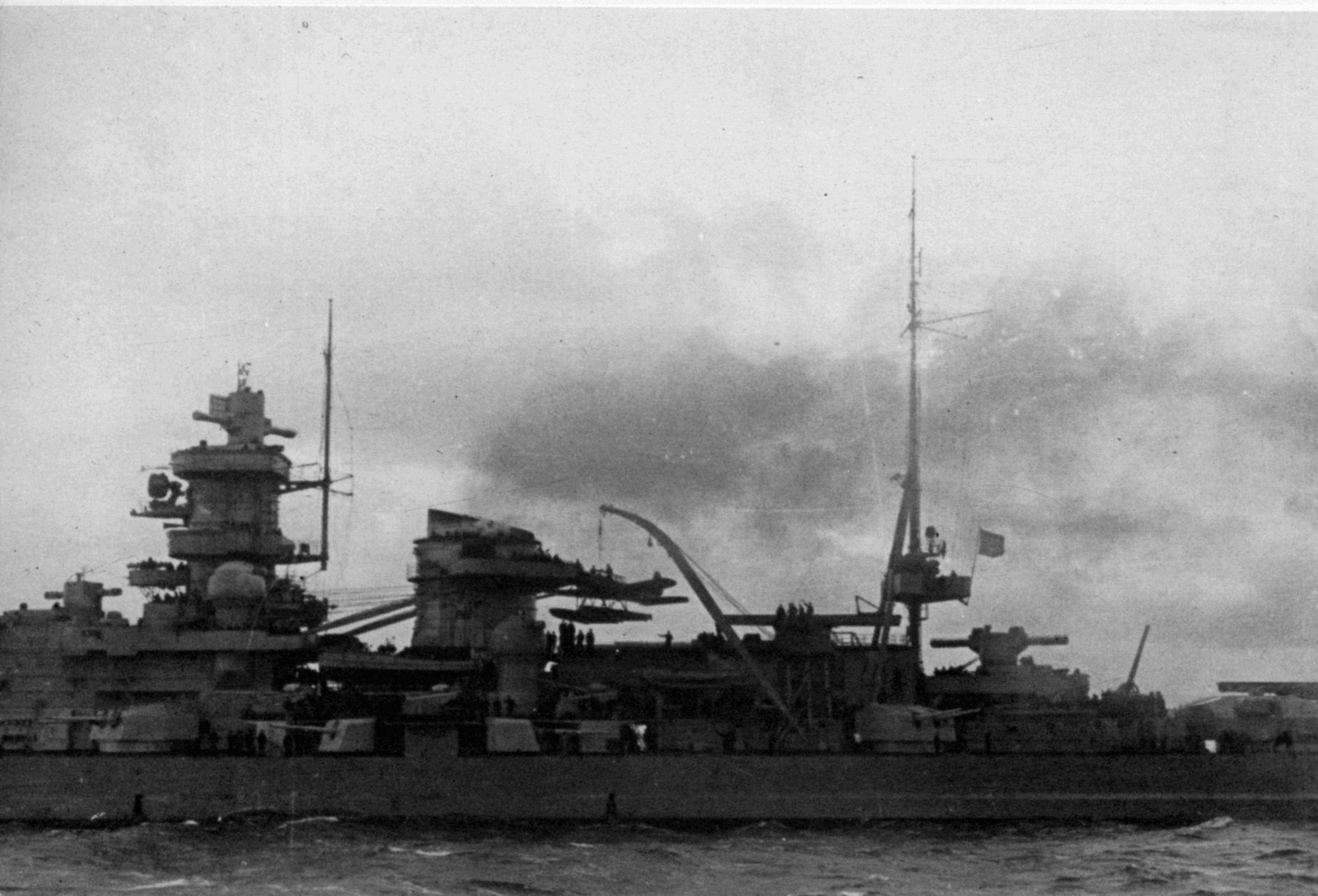
The port aircraft crane lifts an Arado 196 recon. plane aboard. The rotating foretop cover is already fitted with a radar antenna.
