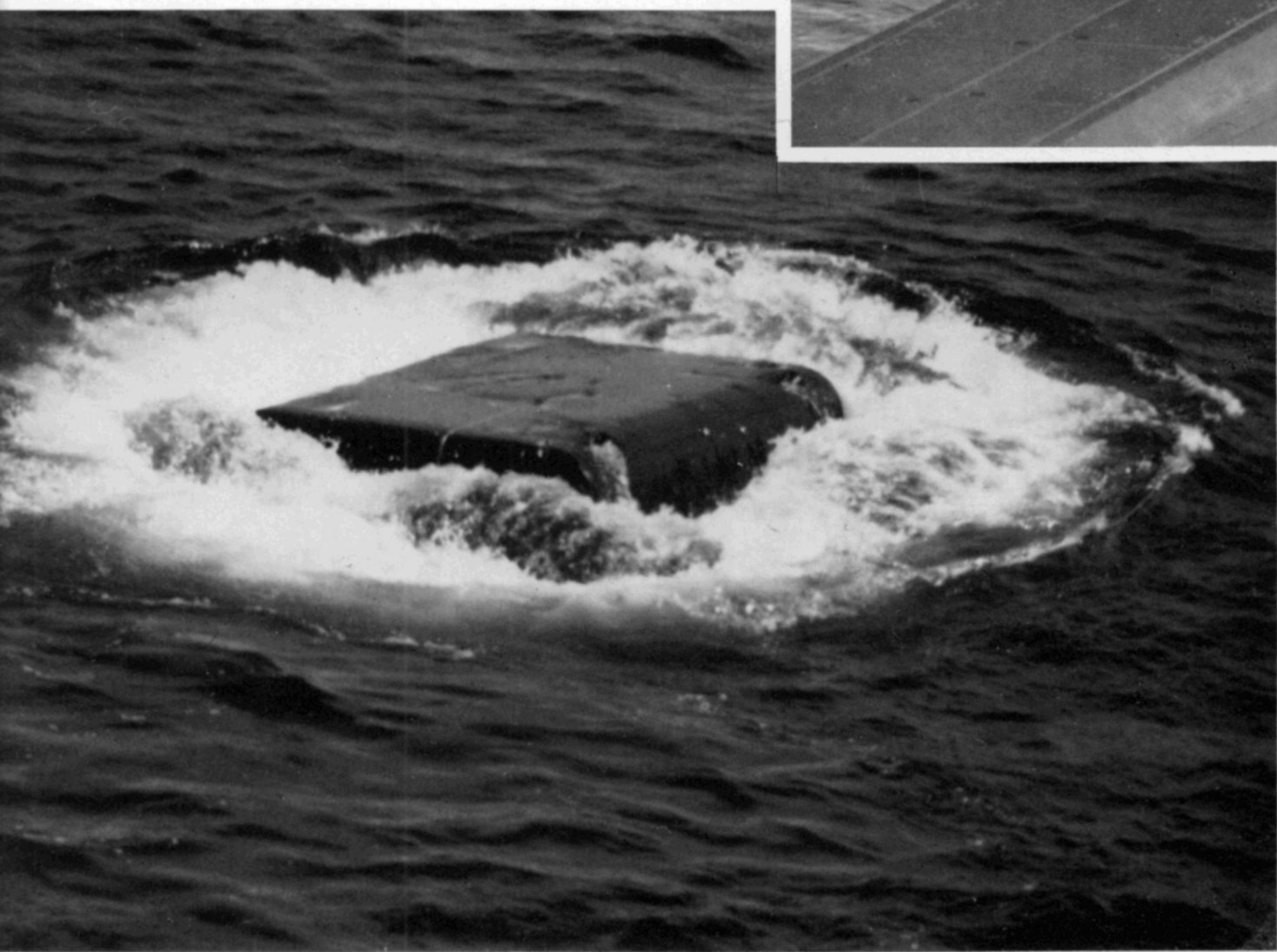
The rescue system in action: From a depth of 80 meters it reached the surface in exactly 58 seconds.
